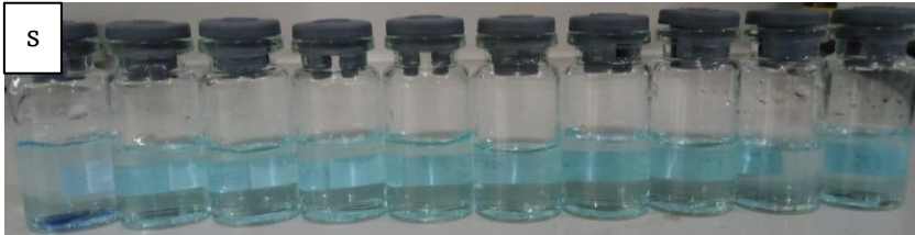
Gambar 10.2 Perbedaan warna ketika fotodegradasi langsung dari menit 0 (kiri) sampai menit 90 (kanan) pada sampel (a) \text{TiO}_2 (b) \text{SMC}_{100} NH (c) \text{SMG}_1 NH (d) \text{SMG}_{10} NH (e) \text{SMG}_{20} NH (f) \text{SMG}_{100} H (g) \text{SMC}_{100} H (h) \text{SMG}_1 H (i) \text{SMG}_{10} H (j) \text{SMG}_{20} H (k) \text{TiO}_2/\text{SMC}_{100} NH (l) \text{TiO}_2/\text{SMG}_1 NH (m) \text{TiO}_2/\text{SMG}_{10} NH (n) \text{TiO}_2/\text{SMG}_{20} NH (o) \text{TiO}_2/\text{SMG}_{100} H (p) \text{TiO}_2/\text{SMC}_{100} H (q) \text{TiO}_2/\text{SMG}_1 H (r) \text{TiO}_2/\text{SMG}_{10} H (s) \text{TiO}_2/\text{SMG}_{20} H
