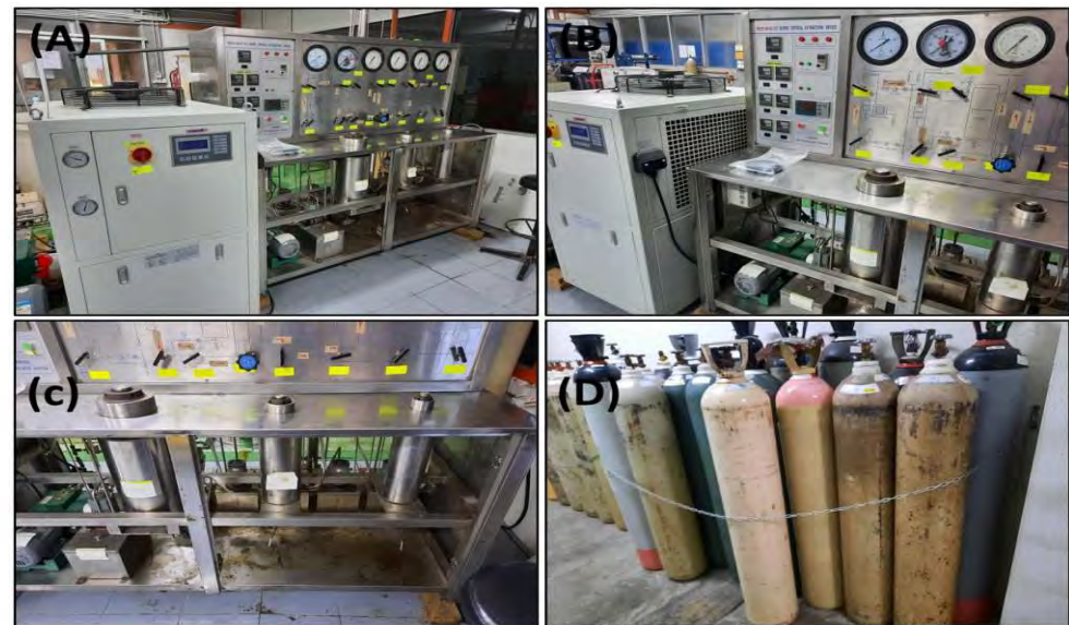
Figure 2: (A) Super Critical Extraction Machine (SFE), (B) Controller of SFE (Pressure and temperature), (C) Sample vessel and two-vessel separators, (D) Carbon dioxide (CO 2 ) tanks
