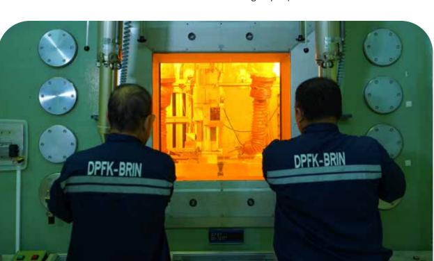
An officer from the Directorate for Nuclear Facility Management (DPFK) at BRIN retrieves an irradiation target in the Hot Cell – G.A. Siwabessy Multipurpose Nuclear Reactor to support Indonesia's radioisotope production sovereignty. Photo © BKPUK
