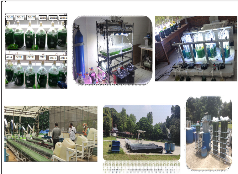
Gambar 4. Beragam jenis konfigurasi PBR indoor bench top bubble column (a) dan indoor hybrid CO 2 biosequester (b), semi out-door membrane PBR (c), PBR adveksi Jungkat Jungkit semi out-door (d), inclined out-door PBR (e), dan Close-loop Vertical out-door PBR (f) (Awalina et al., 2024a; 2024b)
