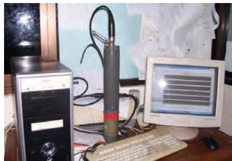
d. Water Quality Logger
