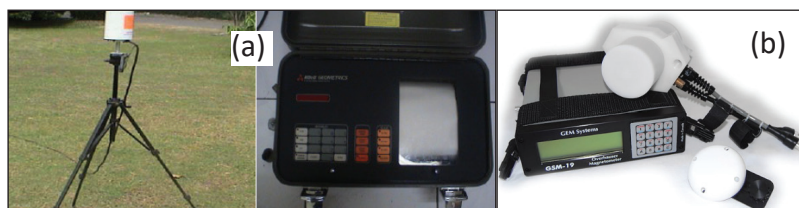
Gambar 6.6 Magnetometer Jenis Skalar
