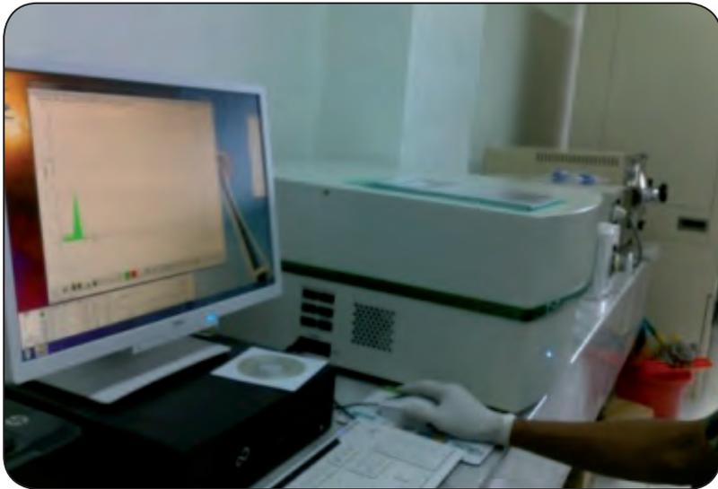
**Gambar 104.** Alat *flow cytometer*
