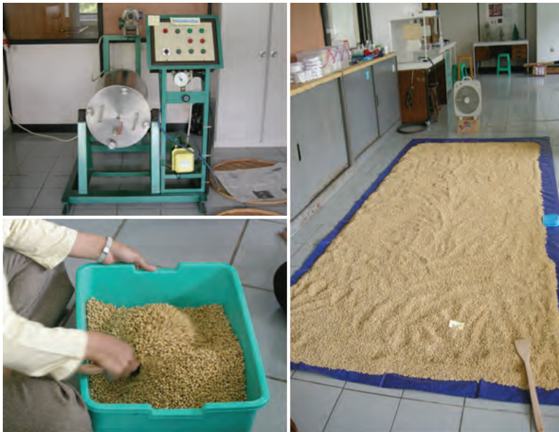
Figure 4. The Application of Technology in the Production of “Soybean Plus” ( Kedelai Plus ) at a Bench Scale with Capacity of 50 kg per Batch
