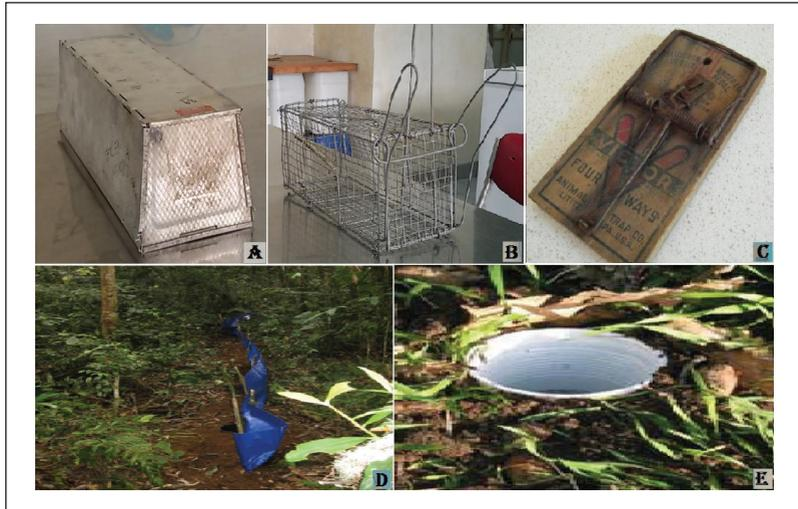
Ket.: A. Sherman trap; B. Kasmin trap; C. Victor snap trap; D. Pitfall line trap; dan E. Single pitfall trap.
