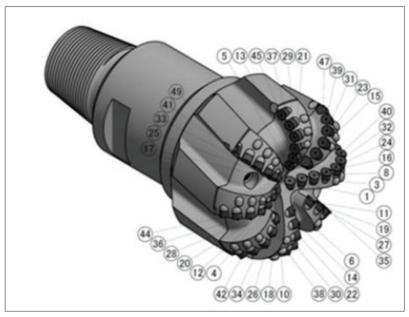
Source: Imaizumi et al. (n.d.) Figure 9.2 D CAD Modeling for 8-1/2" PDC bit
